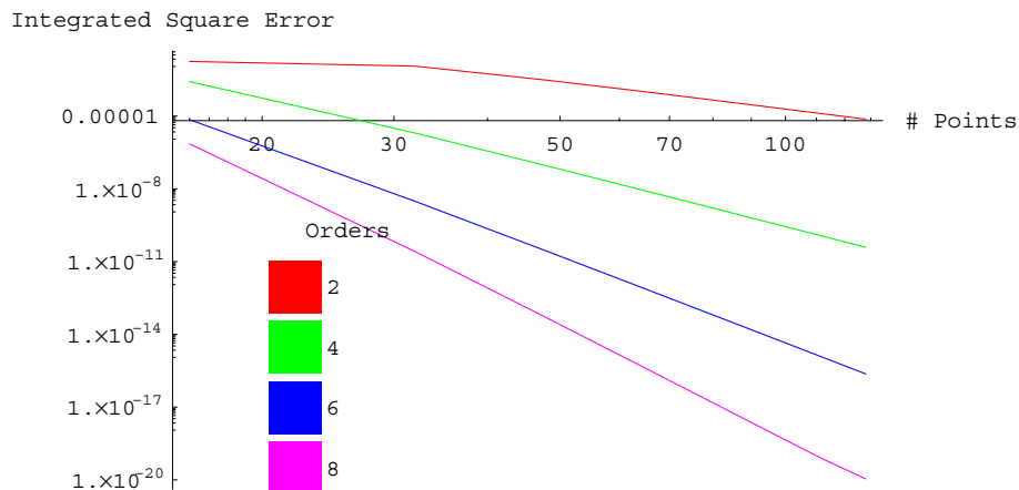
Fig. 3. Integrated square error at t = 1/2 ( N/2 steps) for a square grid, periodic boundary conditions.
